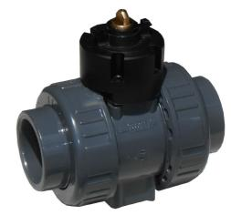
The seal is assured by **two seats in PTFE** with **o-ring in EPDM** (FKM available) to get durability and a soft operation. With the lever on issue, without any special tool, it's possible to **set the tightening** of the seats or to open the valve body for inspection. The pipe unions are **female threaded Gas ISO 228** or smooth, ready **to be glued** to the pipes.
