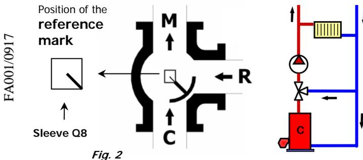
3 ways sector valve, used in mixing, placed on the delivery side; inlet is always a lateral way. Water of boiler (C) is mixed with returning water (R) and sent to the delivery side (M)
