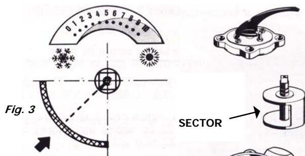
After installing the valve and positioning its rod, the graduated plate (showing the adjustment) has to be placed on the cover. On one side of the plate there is the 0-10 scale, on the opposite side the 10-0 scale.
