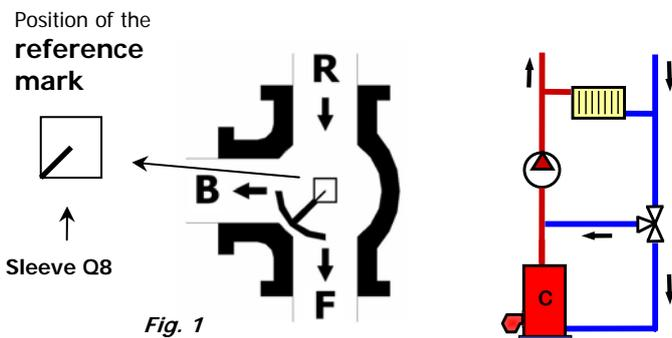
3 ways sector valve, used in deviating, placed on the returning side; inlet is always a lateral way. Returning water of the installing (R) is deviated to the by-pass (B) and ricirculated to boiler (F)
