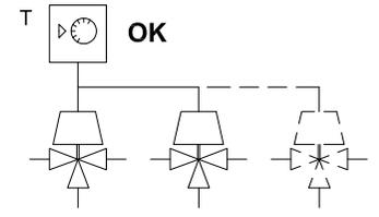
**2 wires** actuators **CAN** be connected in parallel to a single room thermostat / control unit.
