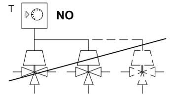
**3 wires** actuators **CANNOT** be connected in parallel to a single room thermostat / control unit.
