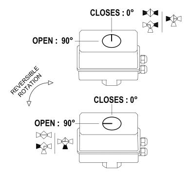
PAY ATTENTION TO THE OPENING AND CLOSING POSITIONS OF THE DE PALA VALVE, REPRESENTED ON THE HEAD OF ITS OPERATING SHAFT, BY A NOTCHED GROOVE IN MODE  $\, \mathbf{I}, \, \mathbf{L} \,$  OR  $\, \mathbf{T}_{\bullet} \,$
