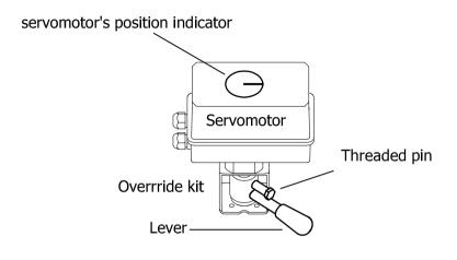
To drive the valve with the servomotor screw the threaded pin completely
