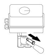
If the threaded pin is locked use 15 mm wrench or move the servomotor forward and backward, switch off the servomotor during manual operations.
