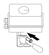
To drive the valve manually unscrew the threaded pin completely
