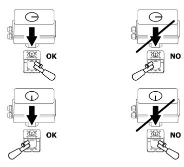
It's possible to assemble the servomotor to override kit spinning it  $90^{\circ}$  /  $180^{\circ}$  /  $270^{\circ}$  compared to the figures above; always pay attention to the related positions before connection.
